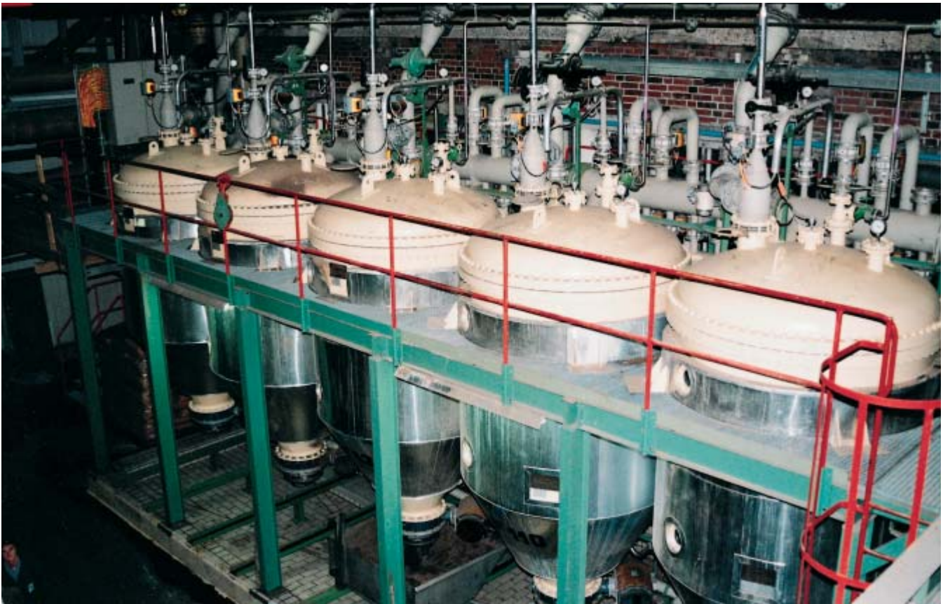
5 FUNDABAC® filters, each 47 m 2 area, vessel carbon steel, hard rubber lined, ø 1900 mm, internal components PVDF, for the filtration of cellulose fibres, yield per cycle 1.5 to solids of 70% dry substance
