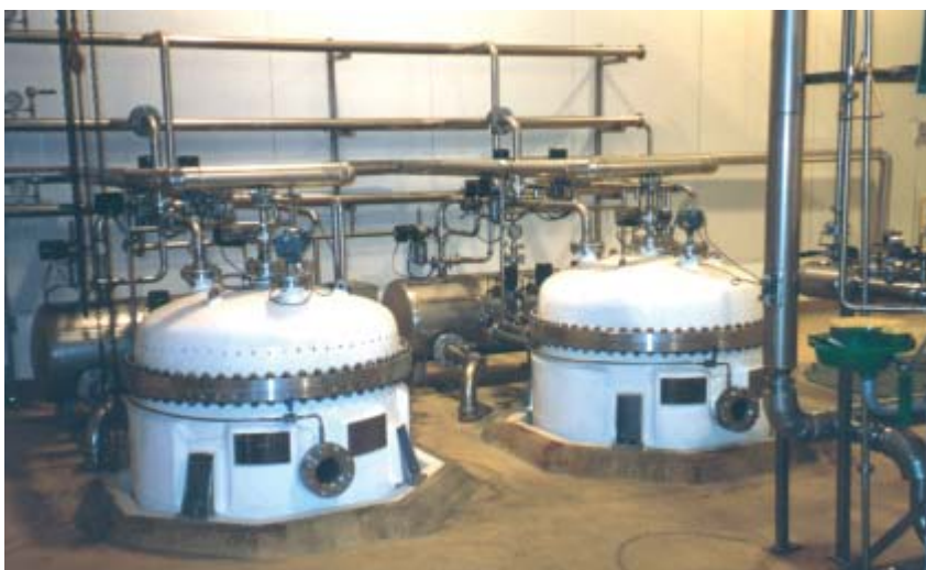
Filters for the production of lactose
